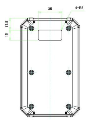
Maximum Carrier Board Dimensions (mm):
