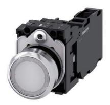
Illuminated pushbutton, 22 mm, round, metal, shiny, white, pushbutton, flat, momentary contact type, with holder, 1 NO+1 NC, LED module with integrated LED 24 V AC/DC, screw terminal
