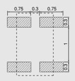
%Note1) The sensor center is located within the  $\phi$ 0.3mm circle. Note2) The tolerances of dimensions with no mentions is  $\pm$ 0.1mm. Note3) Coplanarity:The differences between standoff of terminals are max.50 $\mu$ m.
