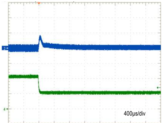
Transient Response ( V_{in}=48\text{V} , I_{out}=2.125\text{A} to 1.06\text{A} , T_a=+25^\circ\text{C} ) Ch2=V out , 200mV/div, Ch4=I out , 1A/div
