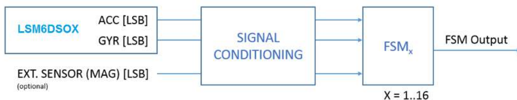
Figure 2. State machine in the LSM6DSOX
