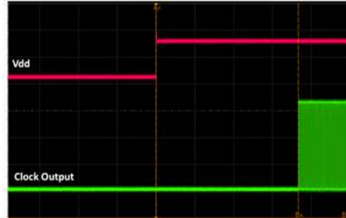
Figure 16. Startup Waveform vs. Vdd
