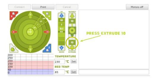
**9B** If you do not see filament coming through the nozzle and the drive gear stops moving, click the **Extrude 10** button once more and wait. Repeat as needed until you see consistent and repeatable extrusion.
