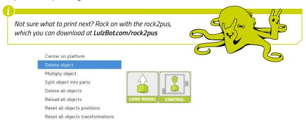
**13E** With your new object set, re-open the Printer Interface window by clicking **Control** in the main Cura interface.
