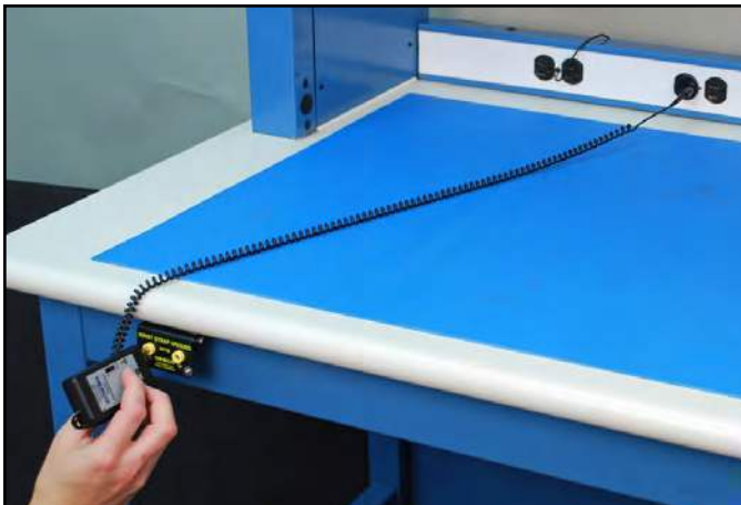
Figure 3. Testing ground points with the 19245 tester
