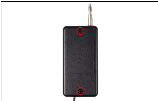
Figure 6. Locating the enclosure screws
