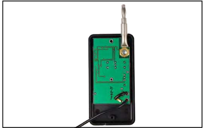
Figure 7. Removing the back cover
