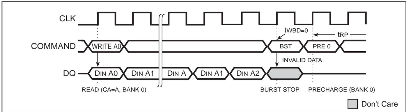
**Burst Data Interruption Using the U/LDQM Pins (Read Cycle)**
