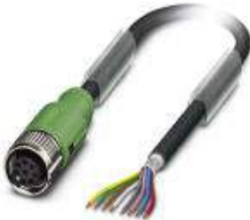
Sensor/Actuator cable, 8-position, PUR, Gray RAL 7001, shielded, Free cable end, on Socket straight M12-SPEEDCON, A-coded, Cable length: 1 m, Twisted pair cables
