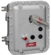
Non-reversing motor starter Size 2 Three phase full voltage Solid-state overload relay OLRelay amp range 13-52a 380-440/440-480V 50/60HZ coil Combination type 60Amp fusible disconnect 60Amp / 600V fuse clip Encl NEMA type 4X Fiberglass Water/dust tight weather proof Standard width enclosure
