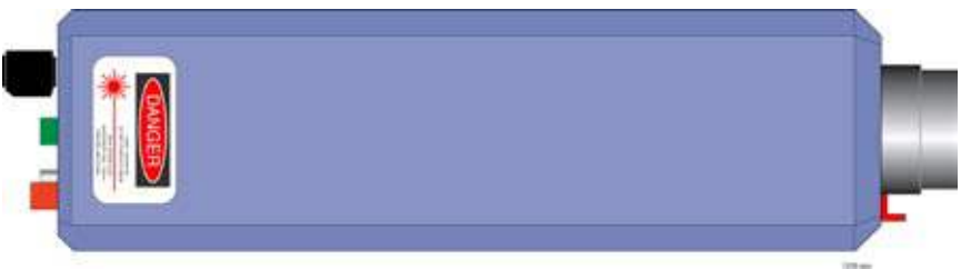
Figure 7. Top view of laser showing the location of the “warning logotype” label for a Class IIIa laser.
