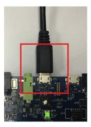
4) Connect the other end of the USB cable to a USB port of the workstation.
