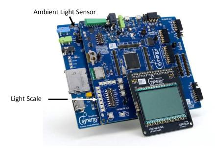
After about 12 seconds, the S3 MCU starts sensing the amount of light at the Ambient Light Sensor, U105. The Demo takes the A/D reading and uses it to display a Light Scale on the Configuration LEDs and as a battery level and digital count on the segment LCD. The elapsed time of the Demo is also shown on the segment LCD.
