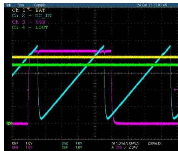
Figure 7. TPS22933A with Varying Inputs and Stable LOUT
