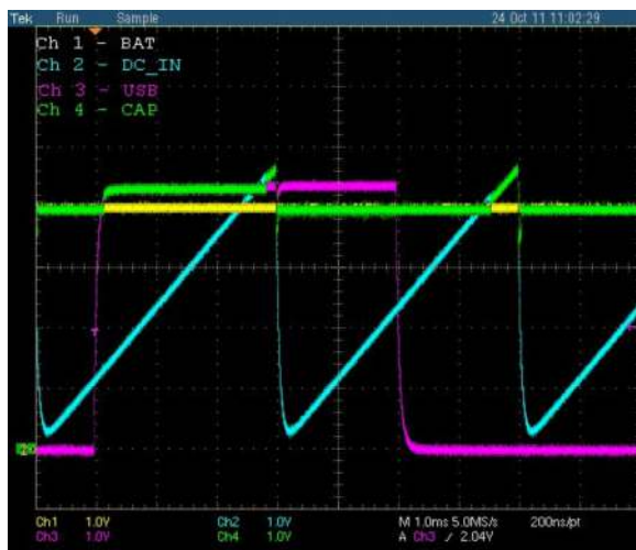
Figure 6. TPS22933A with Varying Inputs and CAP
