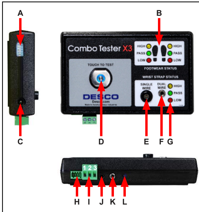
Figure 2. Combo Tester X3 features and components
