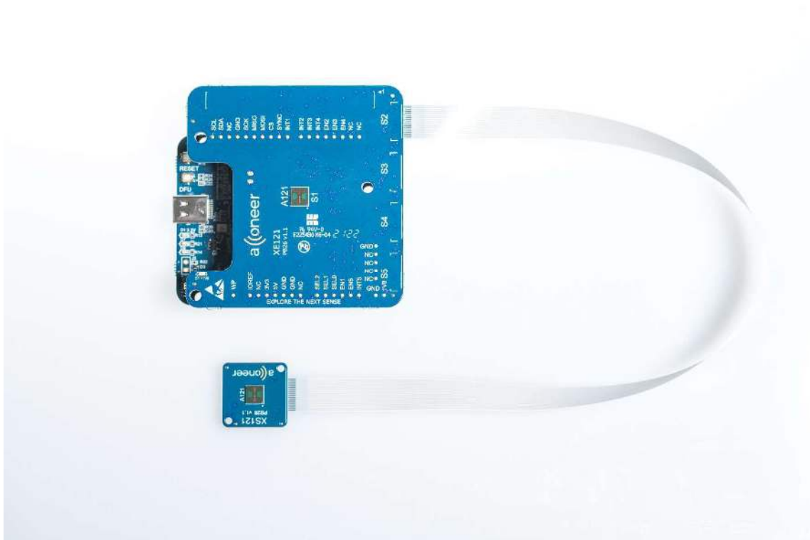
Picture 4. XS121 connected to XE121 which in turn is connected to XC120.
