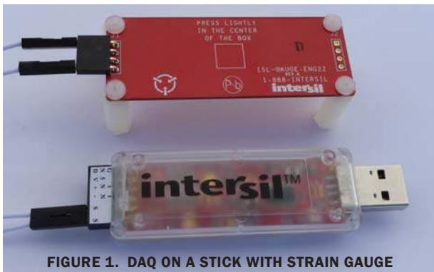
FIGURE 1. DAQ ON A STICK WITH STRAIN GAUGE
