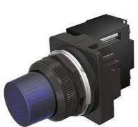
30mm BlackMax, Epoxy Coated Corrosion Resistant Complete Metal Unit Illuminated Indicator Light Full Voltage type, 6V AC/DC LED Lamp, BA9s Glass Lens, Blue UL Listed, CSA Certified NEMA 1,3,3R,4,4X,12,13 & Automotive Standards
