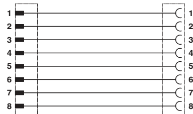
Contact assignment of the M12 connector and the M12 socket
