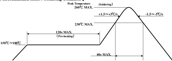
Note 1 Temperature Profile for the reflow should be set to the surface temperature of resin which is on the of LED. This should be the maximum temperature for soldering. Lowering the heating temperature and decreasing heating time is very effective in achieving higher reliability.
