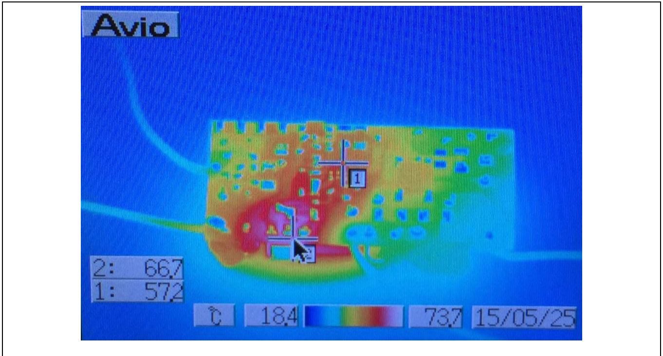
Figure 16 Bottom Side. U1=57.2°C; Q1=66.7°C (66V, 270mA LED load@Vin=230V AC /50Hz)
