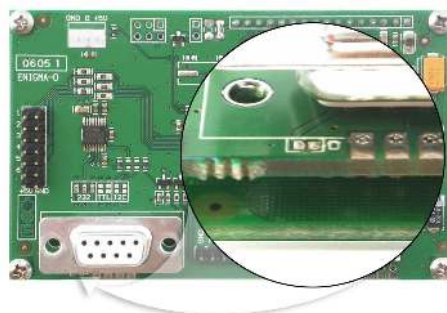
Figure 15: Power Through DB-9 Jumper
