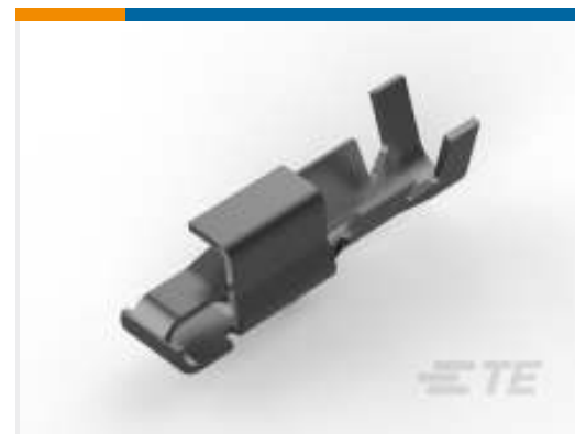
TE Part #3-770522-1 Wire-to-Board Connector Contacts: socket, wire size 30-16 AWG, SL 156
