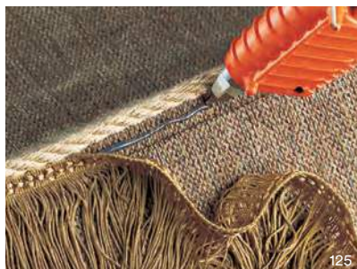
3M™ Hot Melt Applicator LT and 3M™ Hot Melt Adhesive 3792LM applied at low temperature (265°F/129°C) make quick work of wetting, gimping, and bonding fabric to wood.
