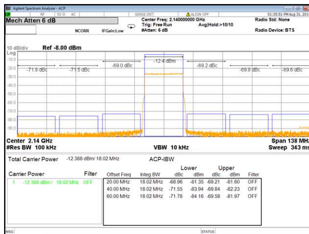
Figure 154. Dual band ACPR Performance in Downlink Band 1 with On-chip PLL
