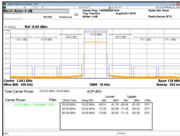
Figure 153. Dual band ACPR Performance in Downlink Band 3 with On-chip PLL
