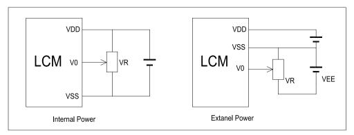
$V_{DD-}V_0$ : LCD Driving voltage VR: 10k~20k
