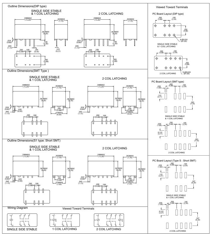
Dimensions in inch with millimeters in brackets below. Tolerance: ± .010"
