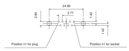
For PCB holes diameters, see on page 1 (finished holes)
