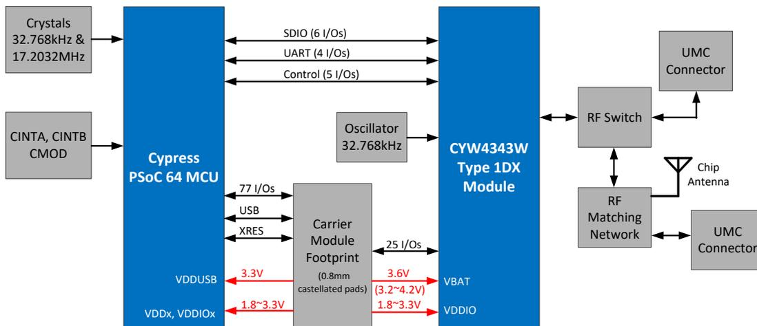
Figure 2-3. Block Diagram of CYW9-BASE-01 Pioneer Board
