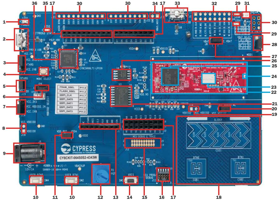
Figure 2-5. PSoC 64 Standard Secure – AWS Wi-Fi BT Pioneer Board - Bottom View
