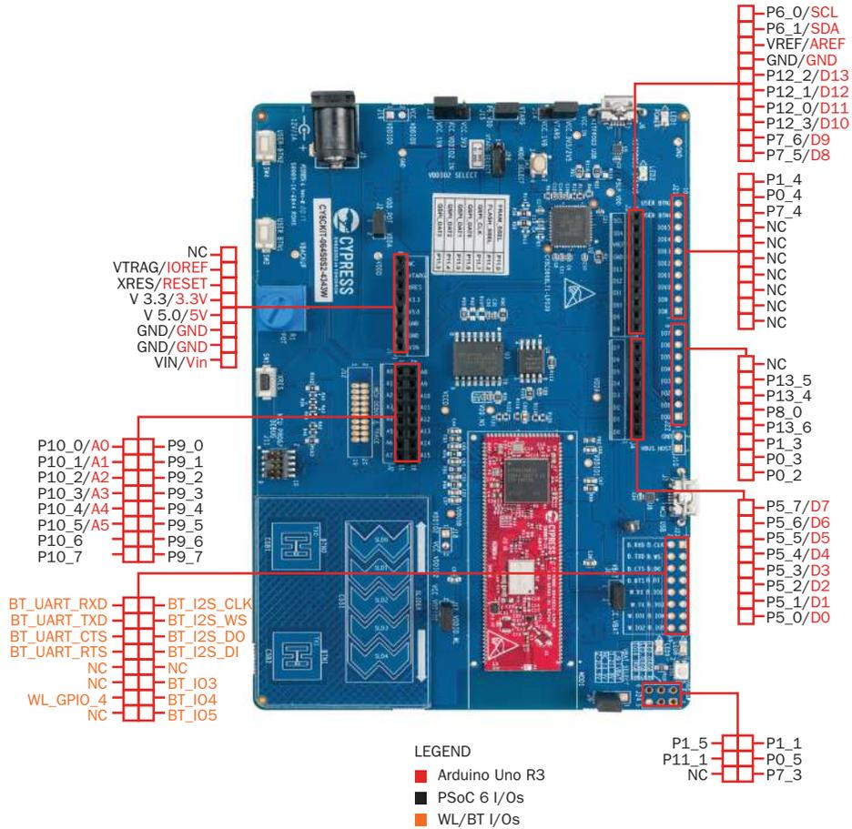
Table 1-1. PSoC 64 Standard Secure – AWS Wi-Fi BT Pioneer Board Pinout
