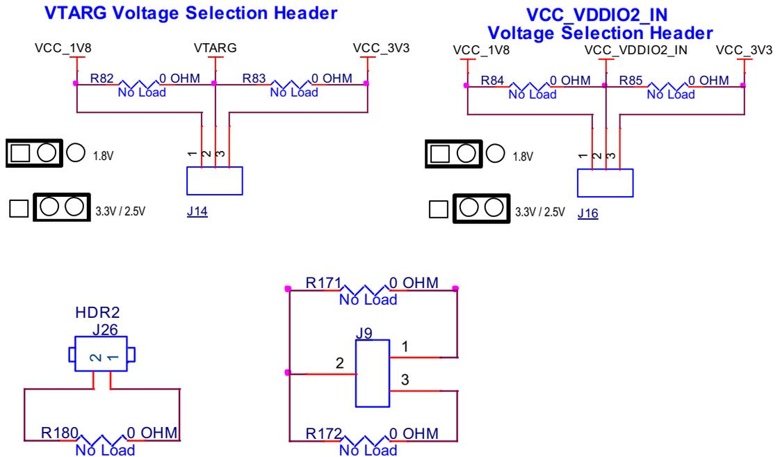
VCC\_VDDIO0 voltage can be selected between VCC\_3V3 and VCC\_1V8 using zero-ohm resistors. It is connected to VCC\_3V3 by default as microSD card (powered by VCC\_VDDIO0) works only at 3.3V. [Figure 4-8](#) shows the schematics of the voltage selection circuits.
