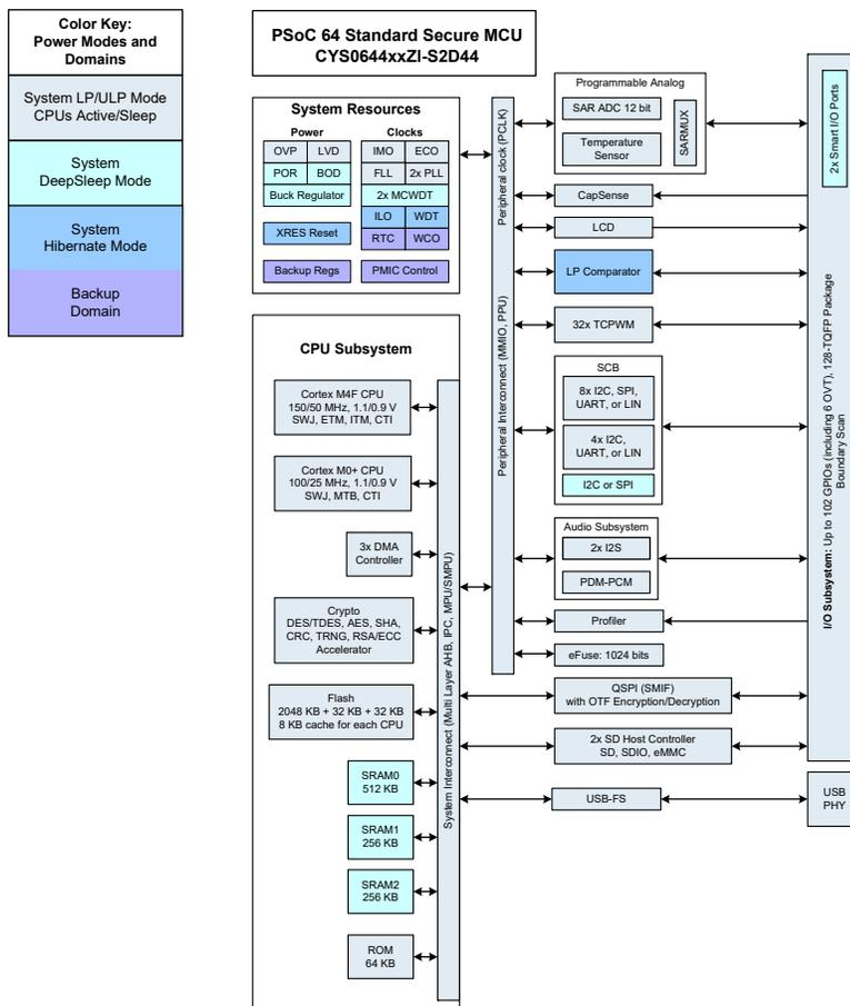
**Note:** PSoC 64 MCU has up to 1024 KB of SRAM; however, 104 KB is reserved for system usage, leaving 920 KB for applications. Similarly, it has up to 2048 KB of application Flash out of which only 1856 KB is usable.
