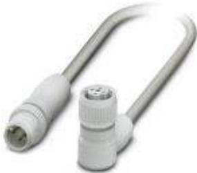
Sensor/Actuator cable, 4-position, PP-EPDM halogen-free, Gray RAL 7035, Plug straight M12, A-coded, on Socket angled M12, A-coded, with 3 LEDs, Cable length: 0.3 m, Hygienic design, with plastic knurl
