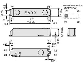
Do not connect #2 and #3 to external device. The metal case inside of the molding compound may be exposed on the top or bottom of this product. This purely cosmetic and does not have any effect on quality, reliability or electrical specs.
