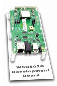
Murata's advanced networking features and robust frequency hopping technology, along with a full 24-bit CRC and ARQ error detection and correction scheme, provide an extremely reliable radio with sophisticated features at a remarkably low price.
