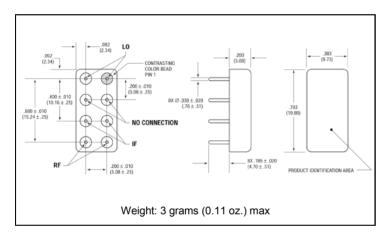
\* Dimensions are inches (millimeters)  $\pm 0.015$  (0.38) unless otherwise specified.
