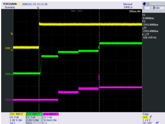
Ch1 – PWM1, PWM2, Ch2 – Vout, Ch3 – Output current (100mA/div)
