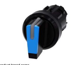
Selector switch, illuminable, 22 mm, round, plastic, blue, selector switch, short, 3 switch positions I>O<II, momentary contact on the left, latching on the right, actuating angle 2x45°, 10:30h/12h/13:30h, with laser labeling, upper case and lower case, always upper case at beginning of line
