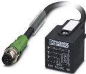
Sensor/Actuator cable, PUR halogen-free, Black-gray RAL 7021, Plug straight M12, A-coded, on A valve plug, with 1 LED, connected with Z diode, Cable length: 0.6 m
