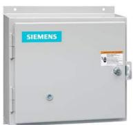
Non-reversing motor starter, Size 0, Three phase full voltage, Solid-state overload relay, OLRelay amp range 3-12a, 24Vdc coil, Non-combination type, Enclosure type 12, Dust/drip proof for indoors, Standard width enclosure
