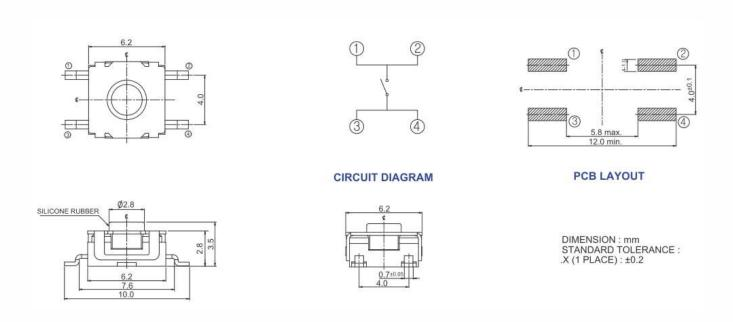
Figure 2 – 222JJV, Surface Mount J-Bend Terminal, Actuator Height 3.5mm
