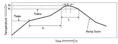
The Pb Free Process-Package Peak Reflow Temperature is 260°C. Exceeding the maximum soldering temperature could permanently damage the module.
