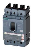
circuit breaker 3VA5 UL frame 250 breaking capacity class C 100kA @ 480V 3-pole, line protection TM230, FTAM, In=90A overload protection Ir=90A fixed short-circuit protection Ii=5...10 x In without connection
