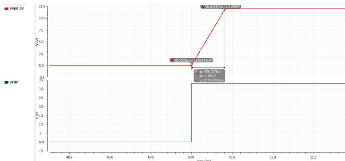
Figure 12. “Standby to normal” operation timing ( C_{\text{REG}} = 1 \mu\text{F} )
