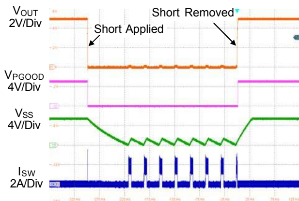
Figure 3. Short Circuit Protection and Recovery
