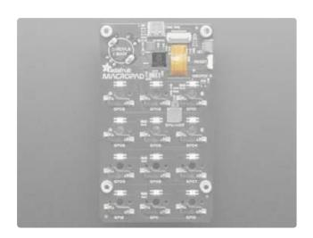
The large square on the back of the board, at the top-center, is the RP2040 microcontroller. This is the brain of the board.
