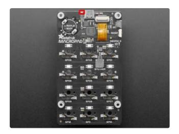
The red LED is located to the left of the USB connector.
