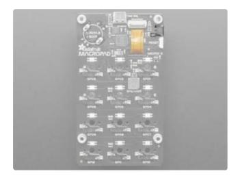
In the top right corner of the back of the board, below the mounting boss, is the STEMMA QT () connector. This Qwiic-compatible I2C connector is designed to make it super simple to connect up STEMMA QT sensors and breakouts ().
