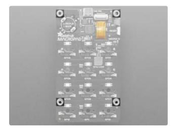
Arranged in the top two corners of the board, and towards the bottom two corners are four mounting bosses to allow for using the MacroPad enclosure kit () or designing your own enclosures.
