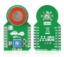
CO click<sup>™</sup> is a simple solution for adding a high-sensitivity Carbon monoxide sensor to your design. The board features an MQ-7 sensor with a SnO2 gas sensing layer, a calibration potentiometer, a mikroBUS™ host socket, two jumpers and a power indicator LED. CO click™ communicates with the target board through mikroBUS™ AN (OUT) line. CO click<sup>™</sup> is designed to use a 5V power supply only.
