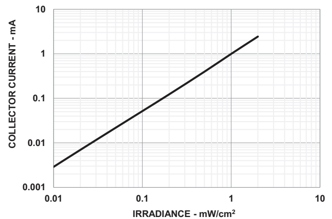
Figure 5: Collector Current vs. Irradiance ( V_{CE} = 5V, \lambda = 940 \text{ nm} )
