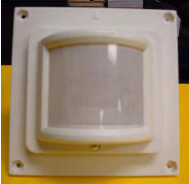
Figure 5. Assembled Flat 1.2" Lens Holder and Flat Lens
