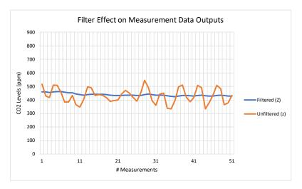
The graph above shows the effects of the filter on the CO<sub>2</sub> measurement data (Z or z). The unfiltered output is shown in orange and the filtered output shown in blue.
