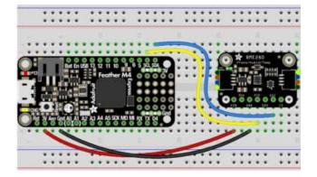
Board 3V to sensor VIN Board GND to sensor GND Board SCL to sensor SCK Board SDA to sensor SDI
