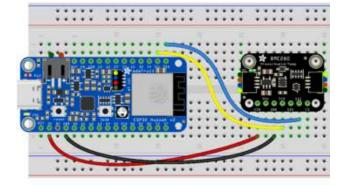
Board 3V to sensor VIN (red wire on STEMMA QT) Board GND to sensor GND (black wire on STEMMA QT) Board SCL to sensor SCL (yellow wire on STEMMA QT) Board SDA to sensor SDA (blue wire on STEMMA QT)
