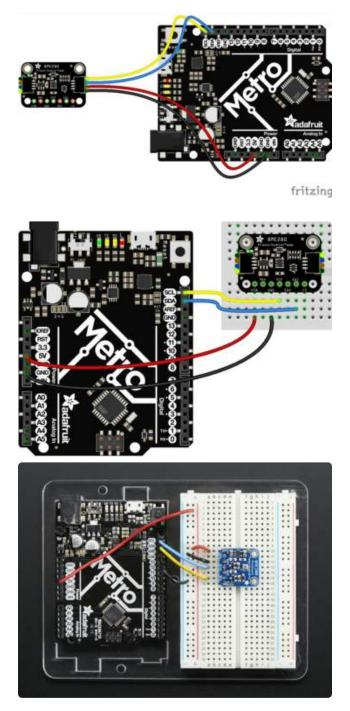
Connect Vin to the power supply, 3-5V is fine. Use the same voltage that the microcontroller logic is based off of. For most Arduinos, that is 5V Connect GND to common power/data ground
