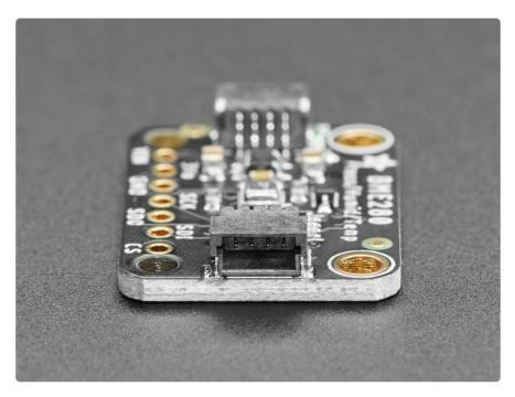
The breakout is made in the <u>STEMMA QT form factor</u> (), making them easy to interface with. The <u>STEMMA QT connectors</u> () on either side are compatible with the <u>SparkFun</u>
