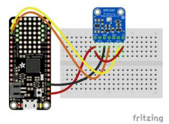
And an example of a Feather M0 wired with hardware SPI:
