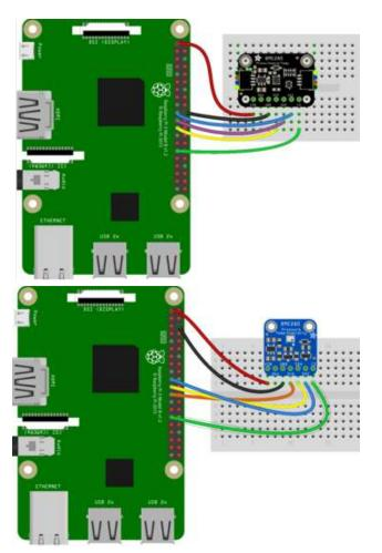
Pi 3V3 to sensor VIN Pi GND to sensor GND Pi MOSI to sensor SDI Pi MISO to sensor SDO Pi SCLK to sensor SCK Pi #5 to sensor CS (or use any other free GPIO pin)
