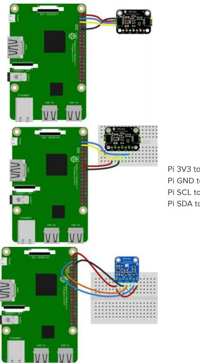
Pi 3V3 to sensor VIN Pi GND to sensor GND Pi SCL to sensor SCK Pi SDA to sensor SDI
