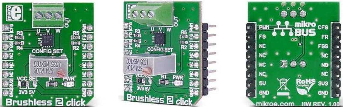
**Brushless 2 click** carries the DRV10964 BLDC motor controller with an integrated output stage from Texas Instruments. The click is designed to run on either 3.3V or 5V power supply. It communicates with the target microcontroller over the following pins on the mikroBUS™ line: AN, RST, CS, PWM, INT.
