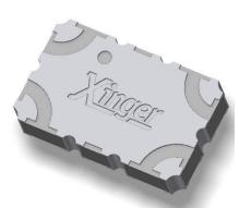
The X3C35F1-04S is a low profile, high performance 4dB directional coupler in a new easy to use, manufacturing friendly surface mount package. It is designed for DC, WCDMA, LTE and PCS applications. The X3C35F1-04S is designed particularly for non-binary split and combine in high power amplifiers, e.g. used along with a 3dB to get a 3-way, plus other signal distribution applications where low insertion loss is required. It can be used in high power applications up to 25 Watts.
